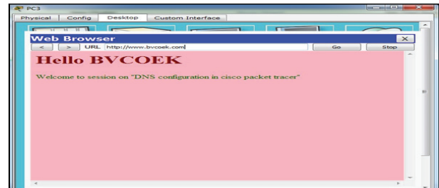
Fig. 20: Type URL: www.bvcoek.com and press enter, Webpage will be opened in PC3
