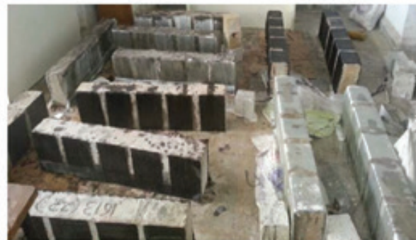
Fig. 2 FRP bonded beams
