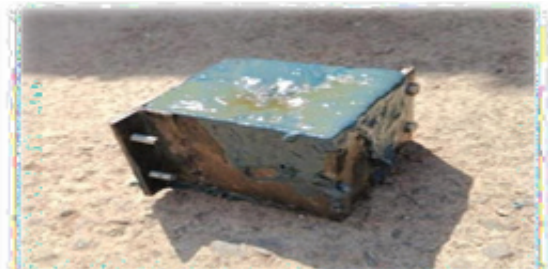
Fig. 6: Molten plastic poured into the mold box
