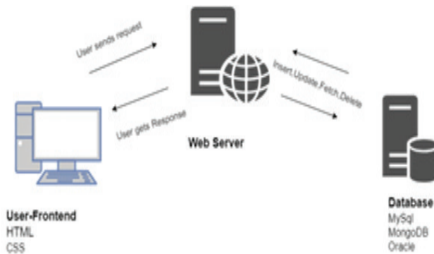
Fig. 2: Backend System Data Transfer
