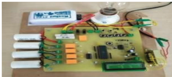
Fig. 6 : Hardware Implemented of APFC-R Load
